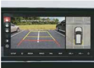
360° CAMERA WITH BVM 4 cameras capture all possible views around the car. Blind View Monitor makes driving in traffic easier.
