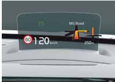
SMART 20.32 CM (8.0") HEAD-UP DISPLAY HUD makes driving safer by minimising the movement of driver's line of sight.
