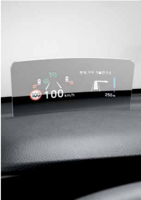
Head-up Display (HUD) As key driving information is projected at the driver's eye level onto the combiner HUD in front of the cluster, it is easier to read navigation data while driving.
