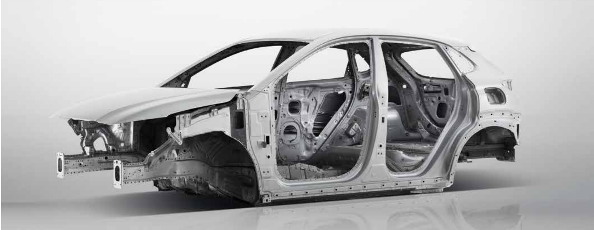
Average strength: 65kgf/mm 2 High Strength Steel is applied extensively to enhance the average body rigidity, safeguard passengers, and ensure driving safety.
