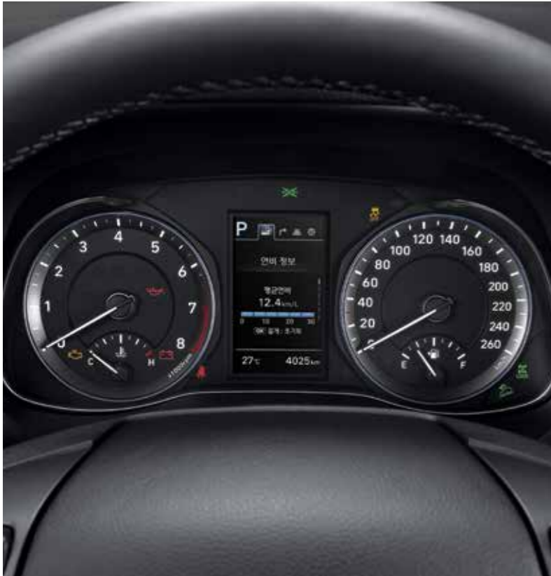
4.2-inch Color LCD Cluster A TFT LCD Cluster helps the driver read key information more quickly while driving with sufficient data via full-color images.
